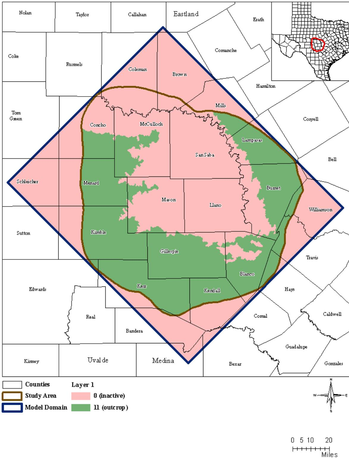
**Figure 2.1.1 Layer 1 active and inactive model cells. Integers in legend are MODFLOW-USG IBOUND values.**
