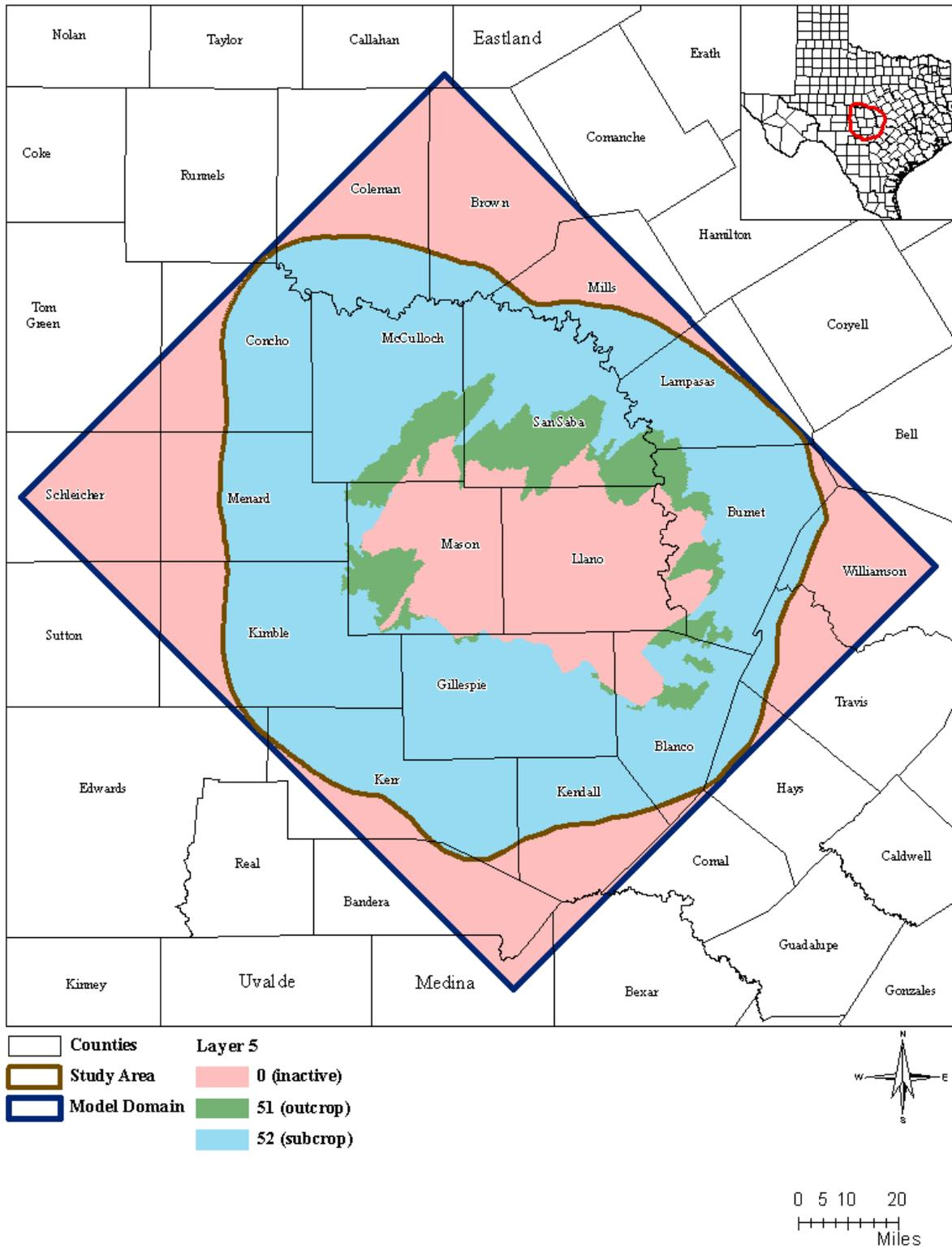
Figure 2.1.5 Layer 5 active and inactive model cells. Integers in legend are MODFLOW-USG IBOUND values.
