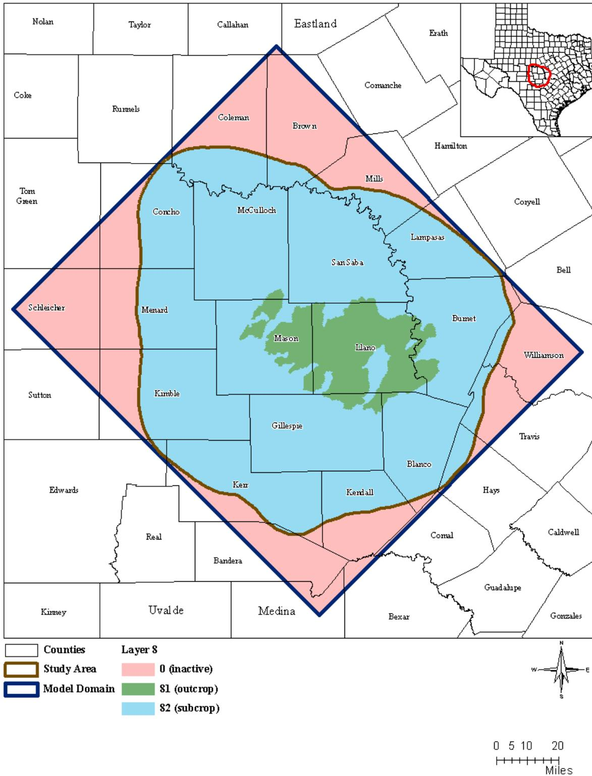
Figure 2.1.8 Layer 8 active and inactive model cells. Integers in legend are MODFLOW-USG IBOUND values.
