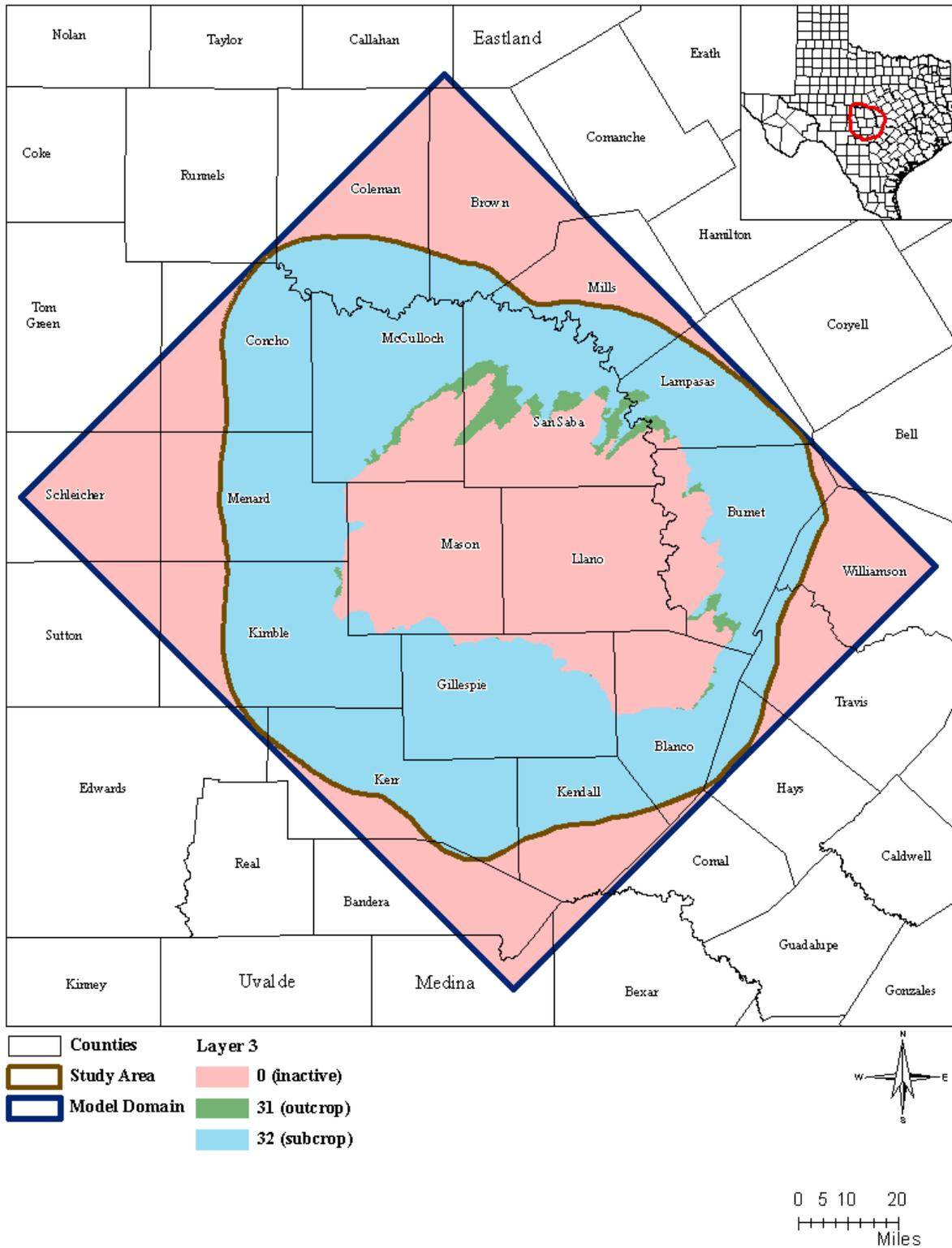
**Figure 2.1.3 Layer 3 active and inactive model cells. Integers in legend are MODFLOW-USG IBOUND values.**
