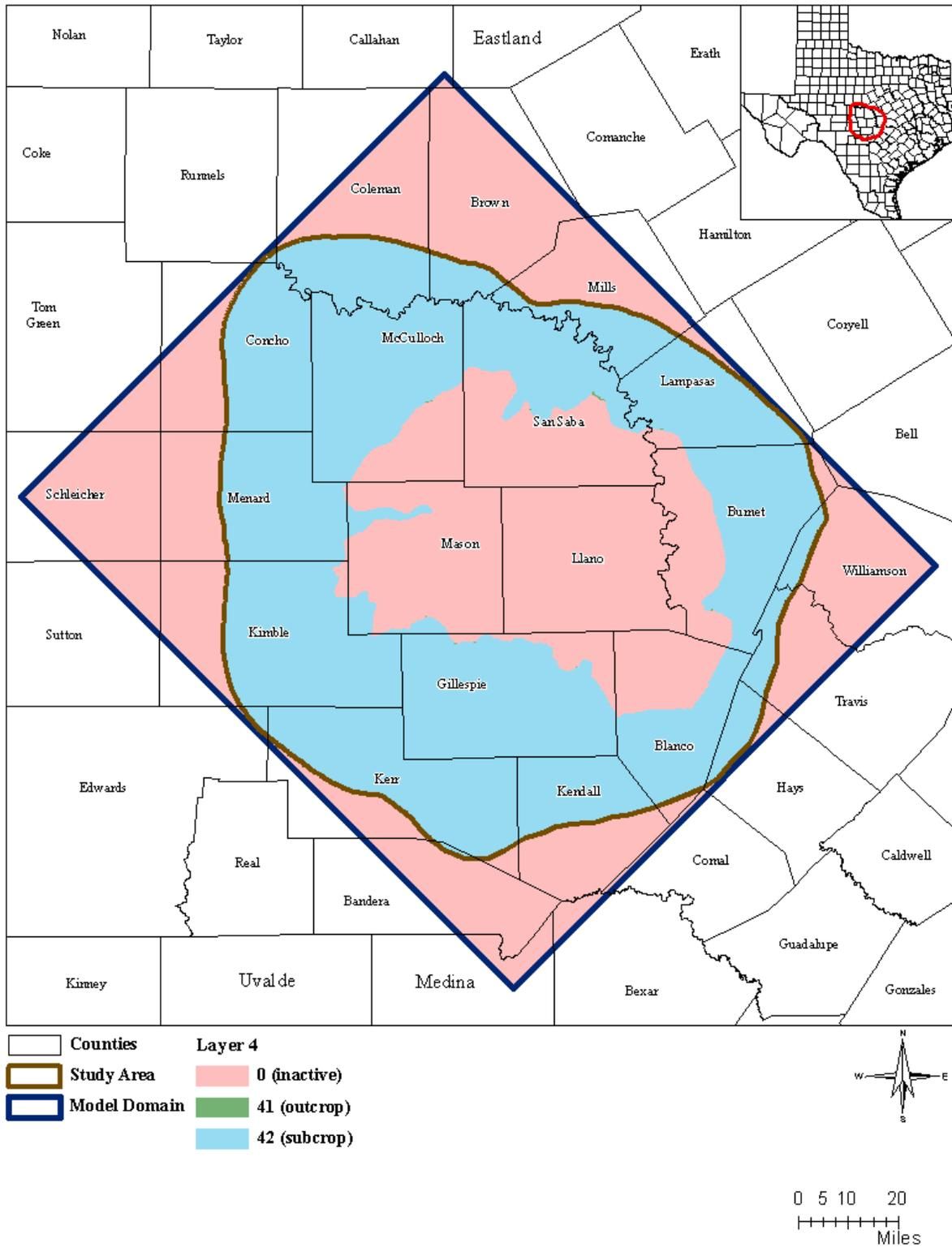
Figure 2.1.4 Layer 4 active and inactive model cells. Integers in legend are MODFLOW-USG IBOUND values.
