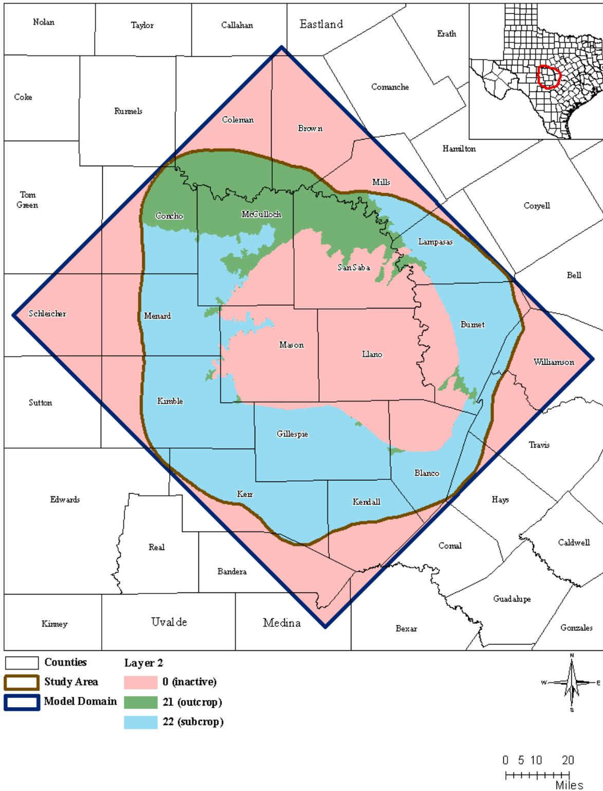
Figure 2.1.2 Layer 2 active and inactive model cells. Integers in legend are MODFLOW-USG IBOUND values.
