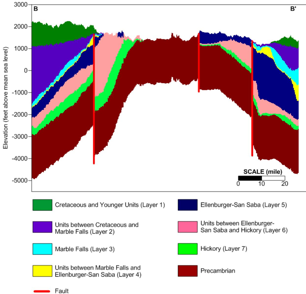
**Figure 2.2.3 Southwest-northeast cross section B-B' along model column 278 (50x vertical exaggeration). Location of cross section is shown in Figure 2.2.1.**
