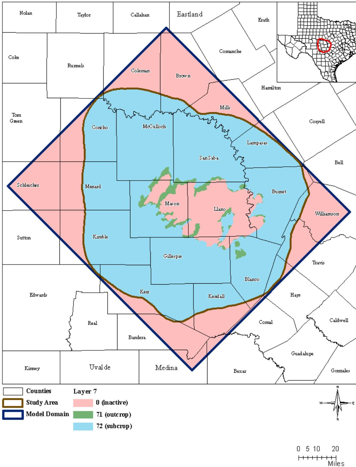
Figure 2.1.7 Layer 7 active and inactive model cells. Integers in legend are MODFLOW-USG IBOUND values.
