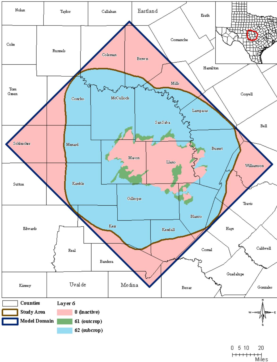
Figure 2.1.6 Layer 6 active and inactive model cells. Integers in legend are MODFLOW-USG IBOUND values.
