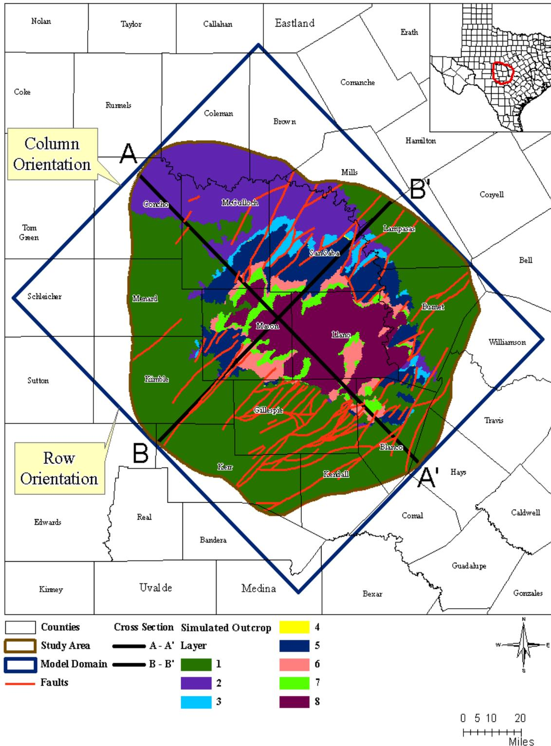
**Figure 2.2.1 Orientation of model grid and locations of cross sections. Model rows are parallel to cross section A-A'. Model columns are parallel to cross section B-B'. Faults are modified from geodatabase by Standen and Ruggiero (2007) with reference to Johnson (2004).**
