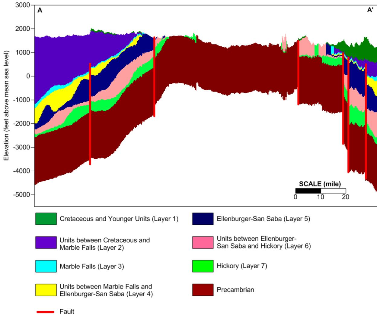
**Figure 2.2.2 Northwest-southeast cross section A-A' along model row 239 (50x vertical exaggeration). Location of cross section is shown in Figure 2.2.1.**
